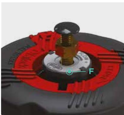
The DKL version of the diaphragm valve is equipped with a handwheel stroke control system which allows the minimum and maximum flows to be preset and preserves the diaphragm from excessive compression during closing operations.
